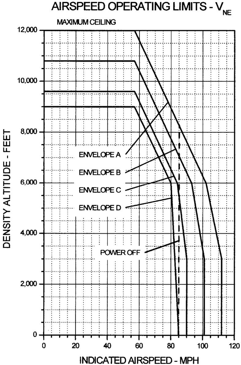
**Figure 5-1.  $V_{NE}$  Variation with Density Altitude**
