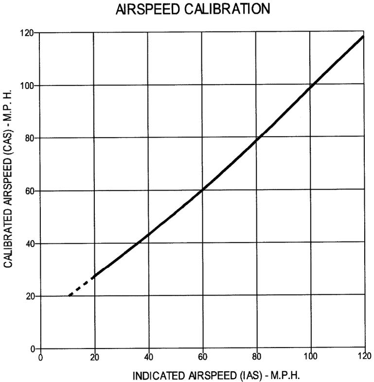
**Figure 5-2. Airspeed Calibration**
