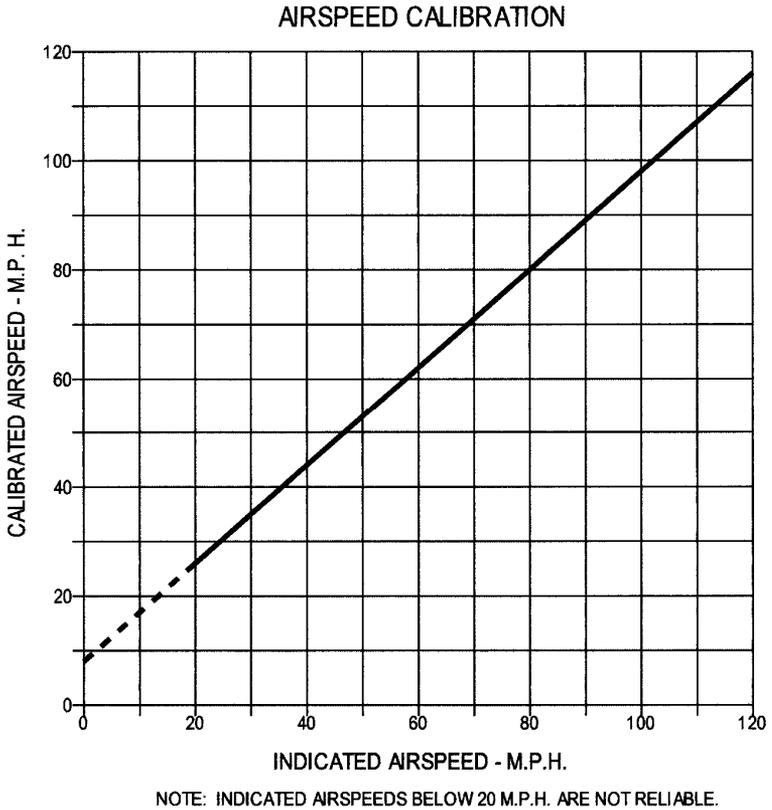
**Figure 10-2-2. Airspeed Calibration Curve w/Float Pitot System (2350 lb)**
