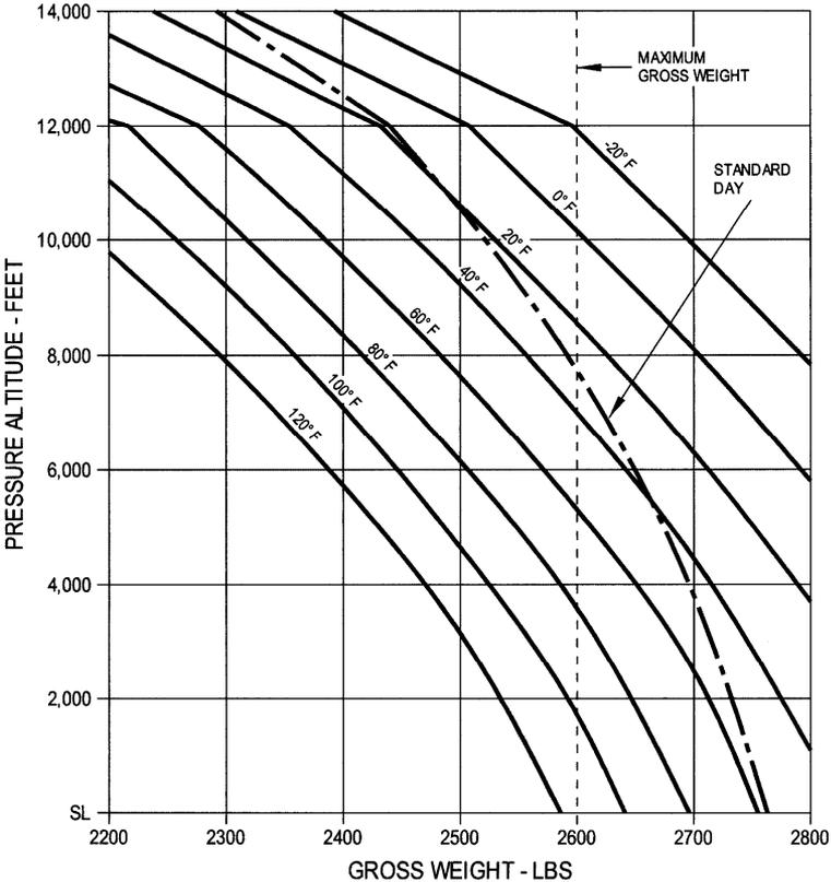
**Figure 5-3. Hover Ceiling In-Ground Effect
