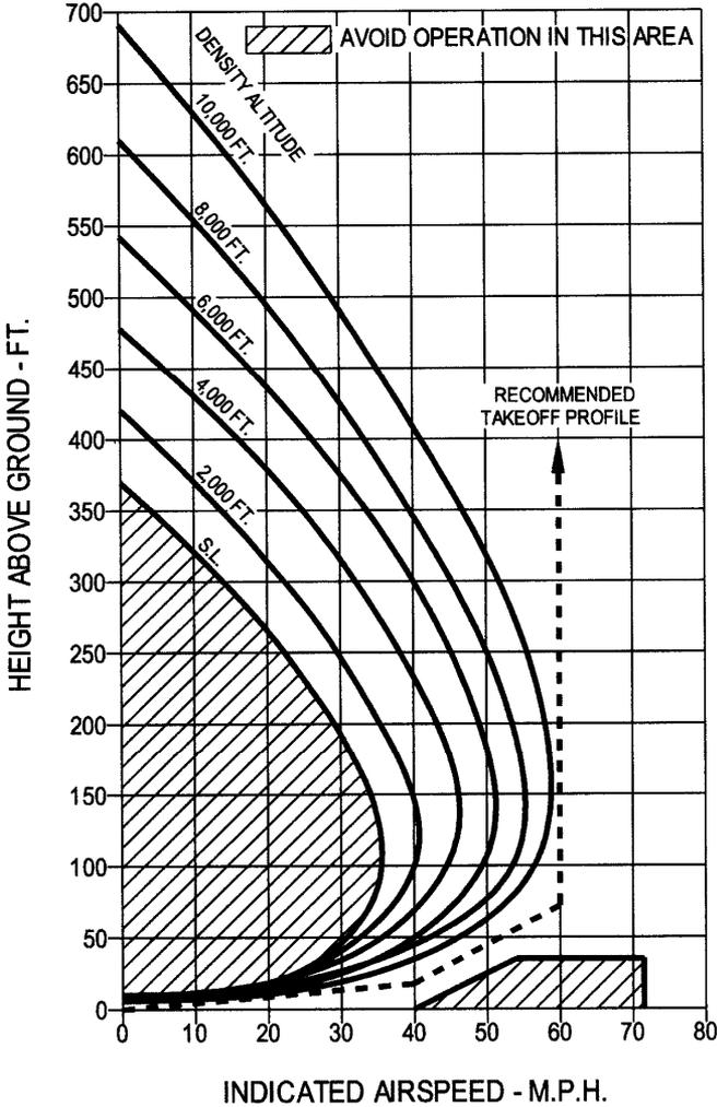
**Figure 5-5. Height Velocity Diagram
