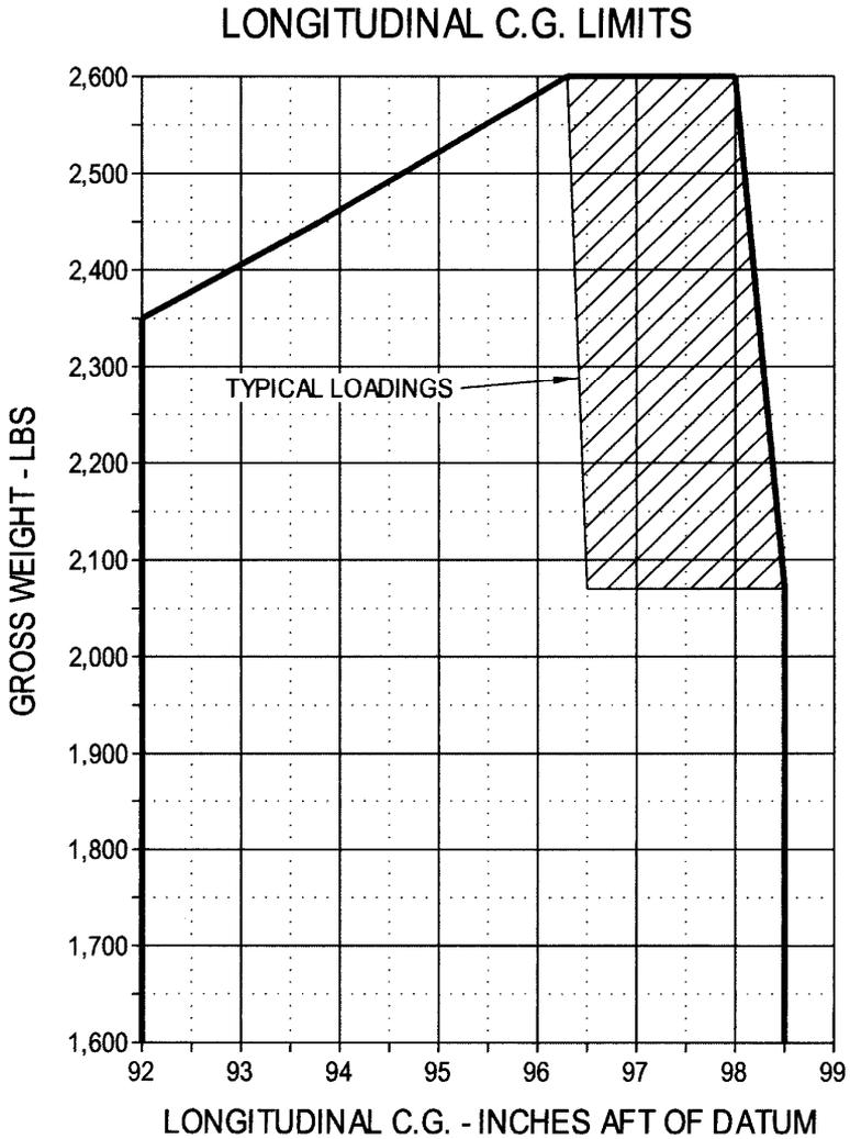
**Figure 10-3-1. Longitudinal C.G. Limits**
