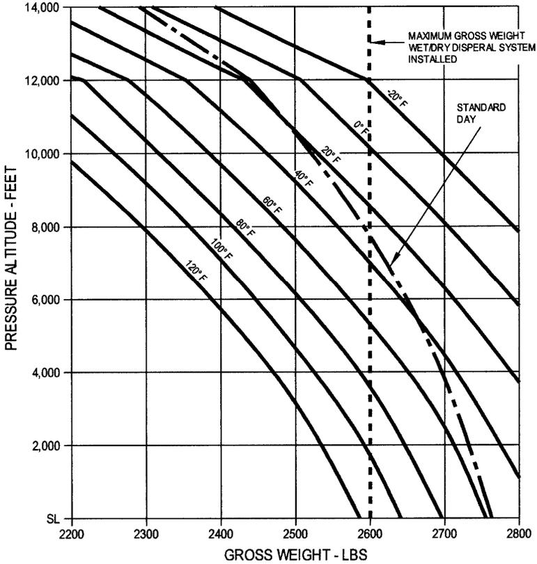
**Figure 10-1-3. Hover Ceiling In-Ground Effect**
