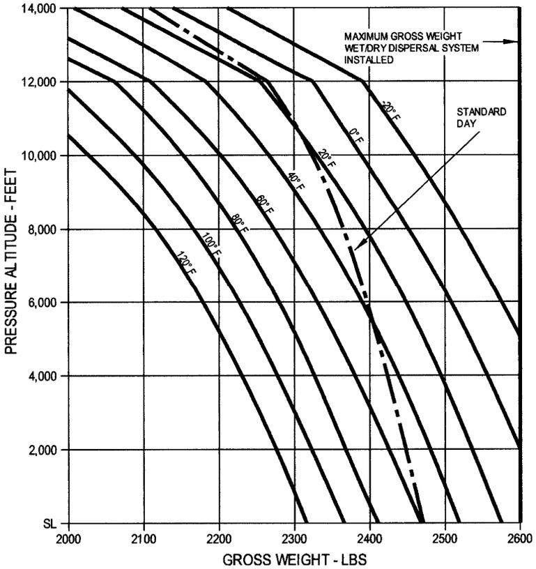
**Figure 10-1-4. Hover Ceiling Out-of-Ground Effect**
