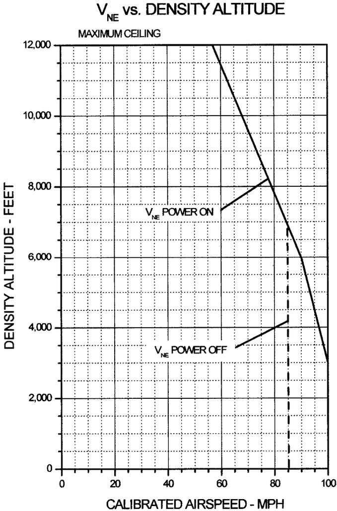
**Figure 10-8-1. V<sub>NE</sub> vs. Density Altitude
