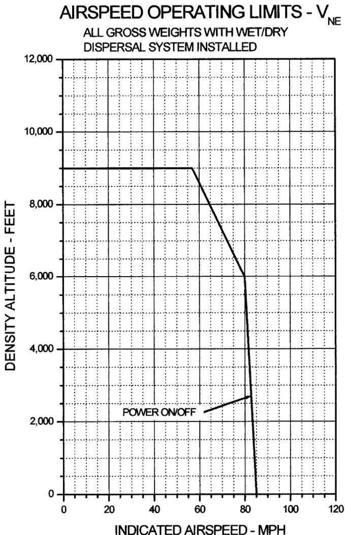
**Figure 10-1-1.  $V_{NE}$  vs. Density Altitude**
