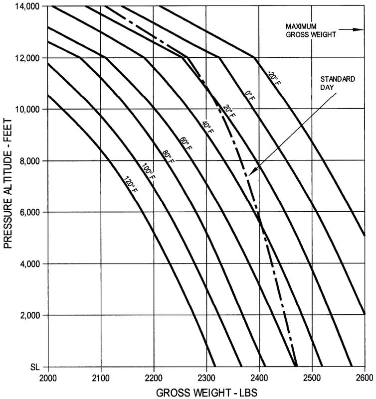
**Figure 5-4. Hover Ceiling Out-of-Ground Effect
