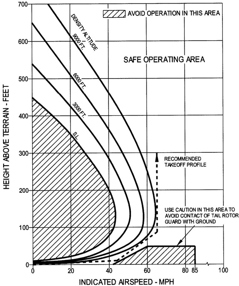
**Figure 5-7. Height Velocity Diagram
