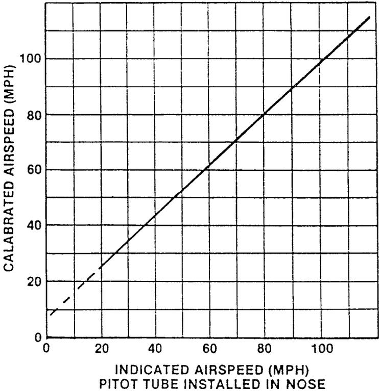
**Figure 10-8-2. Airspeed System – Calibration Curve
